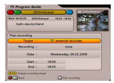
Use the buttons to select the desired recording mode. The recording mode options available are:
